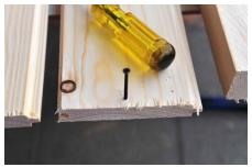
Layout 2 short and 2 long boards to form a rectangle so there is one screw located in each corner.
