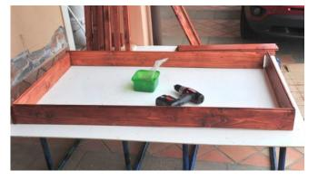
Place the pieces together screw together to form two large rectangles. Be careful to make sure the edges are even before you screw it into place. (Do this on a flat surface to ensure the bottom is level) Don't worry if it seems a little flimsy, as the screws are just to hold it together for you can place the rectangles on top of each other to install the legs.
